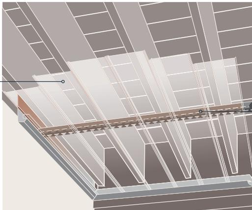
The specially designed panels and deep water brackets have been tested and approved to handle over 15" of water an hour.
